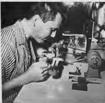
SMALL ELECTRIC motor powers this tiny jeweler's lathe, left, and a sewing machine, right, but a unique air-driven motor, center, is more controllable for laboratory use. An air-driven motor offers precise speed control in critical applications.
